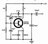
In the Radio Amateurs Handbook, we found a good transistor crystal-oscillator circuit. We built the oscillator circuit on a small pc board and "stole" the required power from the solid-state r-f generator we were using.
